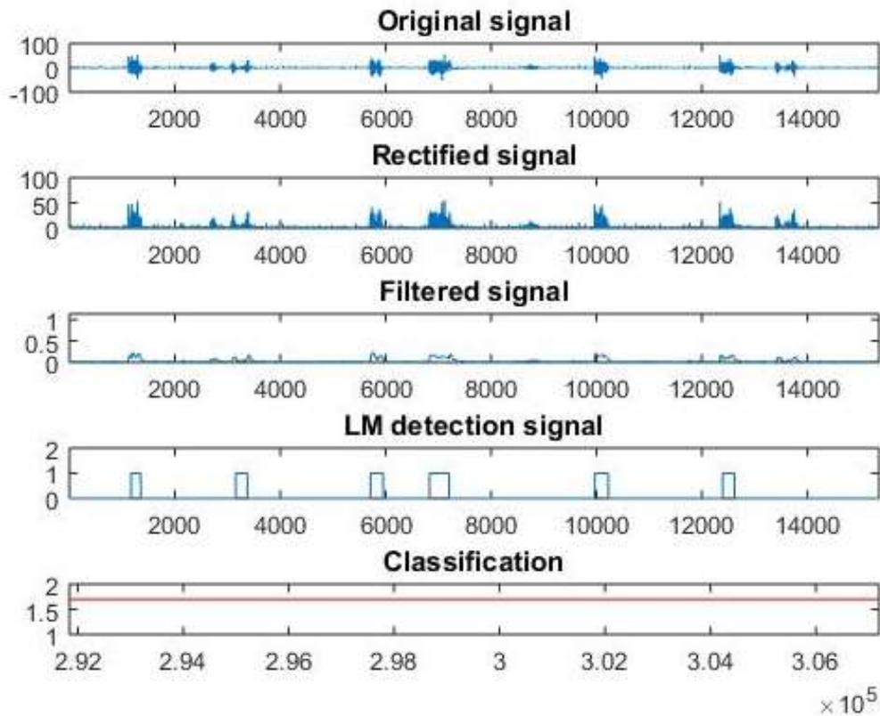
Figure 3. Comparison of the EMG signal of the sample 17853A-C within the different steps of the algorithm: rectifying, filtering, LM detection and movement classification. The length of the interval observed is of 120 seconds.
