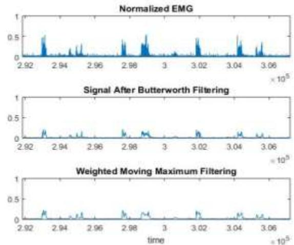
Figure 2. Normalized signal, signal after applying the Butterworth filter and signal after applying the weighted moving maximum filter within an interval of 120 seconds.
