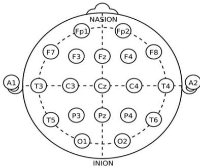
**Figure 3.** Representation of the 10-20 System for the electrode positioning.
